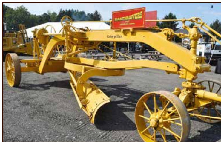
Equipment from yesteryear: construction machinery was on display, including this vintage pull-type Caterpillar grader on loan from Earthmovers Inc. of Danbury, CT.
